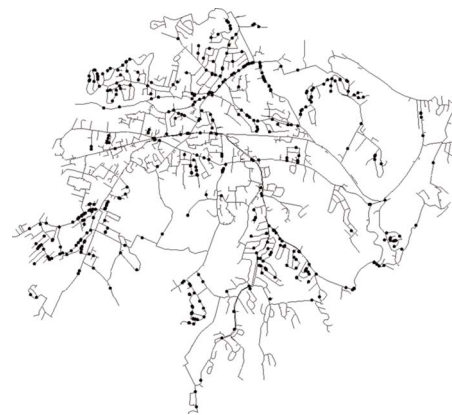
Fig. 2. Drinking water distribution system analyzed in this paper; dots are breaks and lines are pipes
