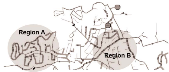
Fig. 4. Two similar groups of pipes (both consisting of 6-in.-diameter, 50-year-old, cast-iron pipes), represented as the dark thicker segments, which have visually different intensity of pipe breaks
