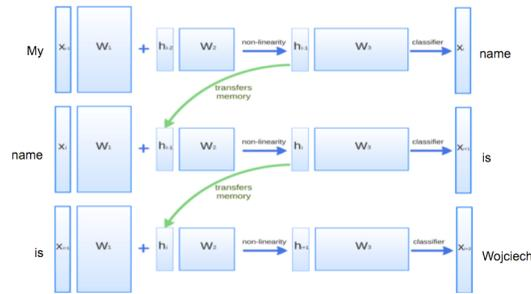
Figure 1.4: Language modelling task. The RNN tries to predict probability of a word given the hidden state  $h$ . The hidden state  $h$  can encode arbitrary information about the past that is useful for the prediction.
