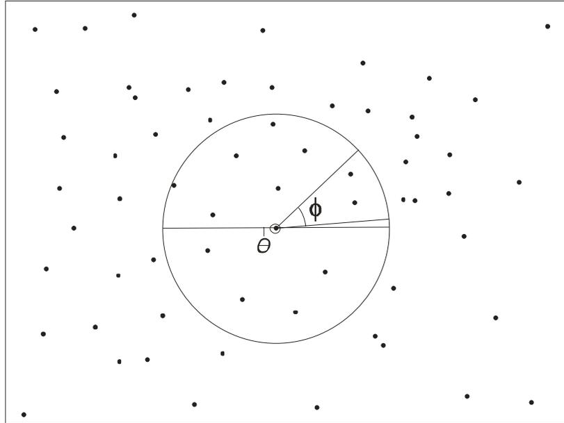
**Figure 13:** A circular region with diameter equal to the image angle parameter  $\theta$  is used to determine a set of ‘nearby’ stars. A wedge is constructed according to wedge angle  $\phi$ .
