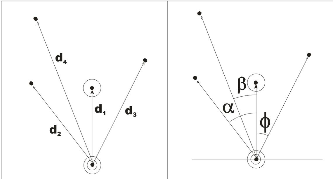
**Figure 15: The two pieces of indexed information are represented. On the left, the distance of stars from the central star. On the right, the angles of the stars relative to the orienting star. In each image, the star of interested is double-circled, and the orienting star is single-circled.**
