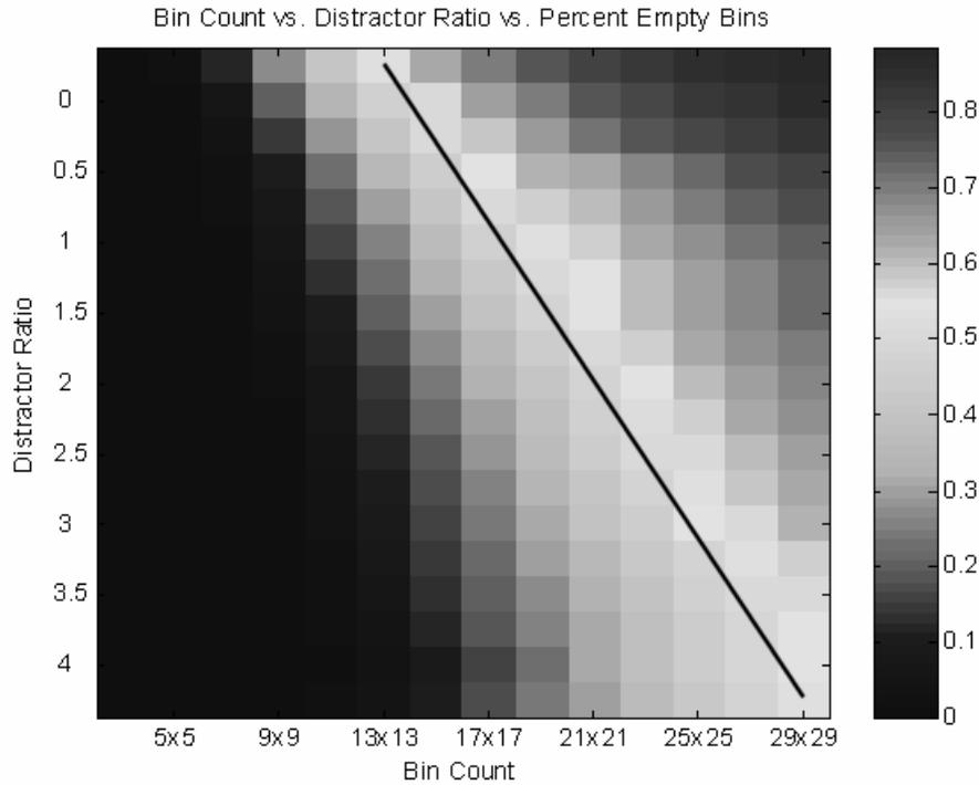
**Figure 8:** An image of the average proportion of empty bins found in the test images according to each binning size. The dark line roughly marks where the bins are 50% empty. The distractor ratio refers to the average proportion of distractor stars in an image relative to catalog stars. So, given an image with 100 catalog stars, where the distractor ratio is 4.0 we would expect an extra 400 distractor stars to be present.
