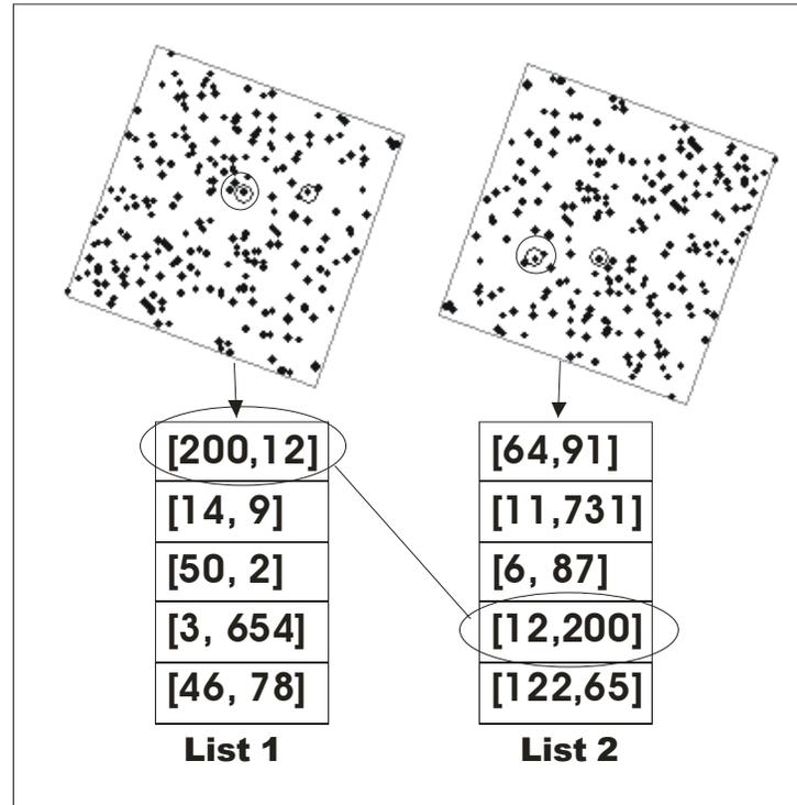
**Figure 3:** An image of the double matching process. The same image and the same pair produce two different solution lists depending on which star centers the grid (the double-circled star) and which lies along the x-axis (the single-circled star). A good solution should appear in both lists with the order of the pair reversed.
