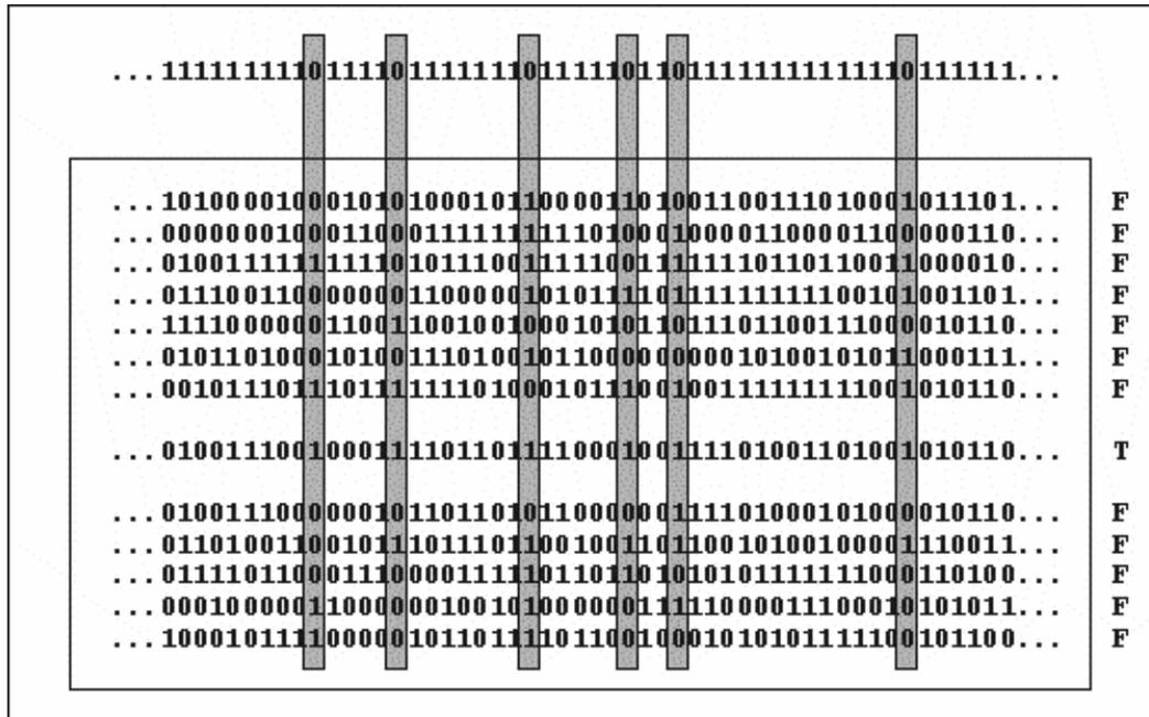
Figure 4: An image representing the matching process of an image code (at top) against indexed codes using a logical-or operation. Codes that, when or'd with the image code, result in no zeros are solution candidates and result in a T (or true) result. Codes that result in one or more zeros fail.
