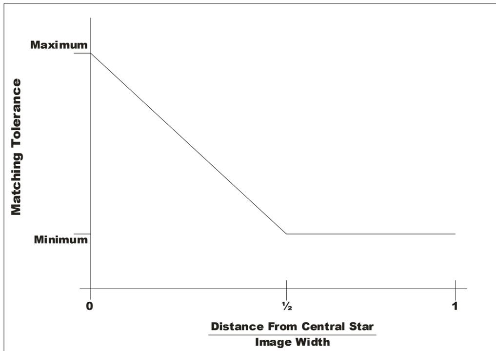
Figure 17: The change in matching tolerance as the distance to the central star increases (distance being measured relative to the width of the image).
