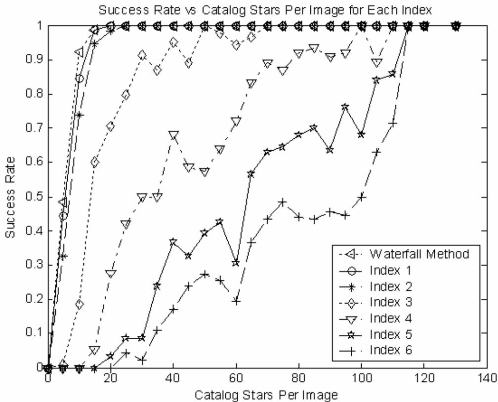
**Figure 20: A plot of the change in success rate for different numbers of catalog stars per image. The numbered indexes refer to the indexes described to at the beginning of Section 3.6. The waterfall approach refers to the process of using all the indexes together.**
