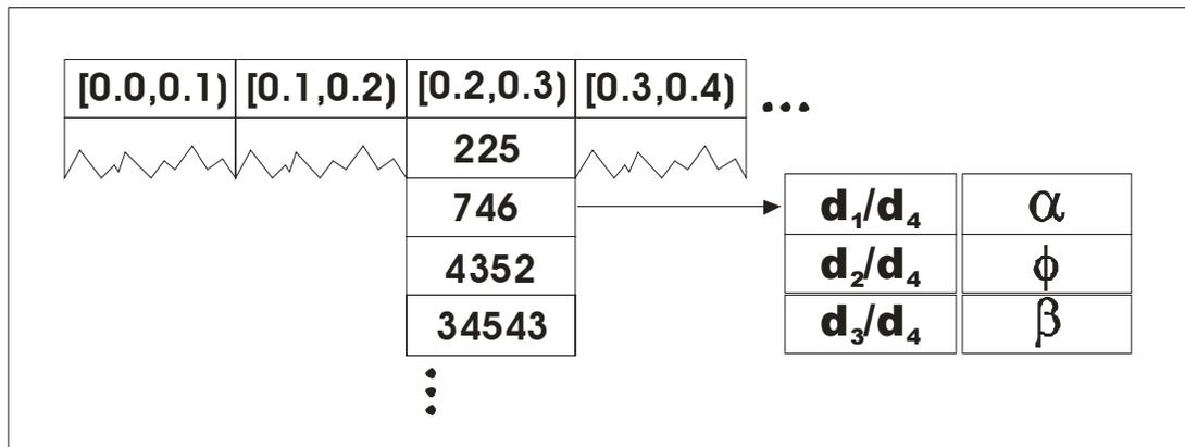
Figure 16: A diagram of the index layout. A lookup table contains shape ID's, which point to a list of distance ratios and angles, sorted from nearest to farthest from the central star of interest.
