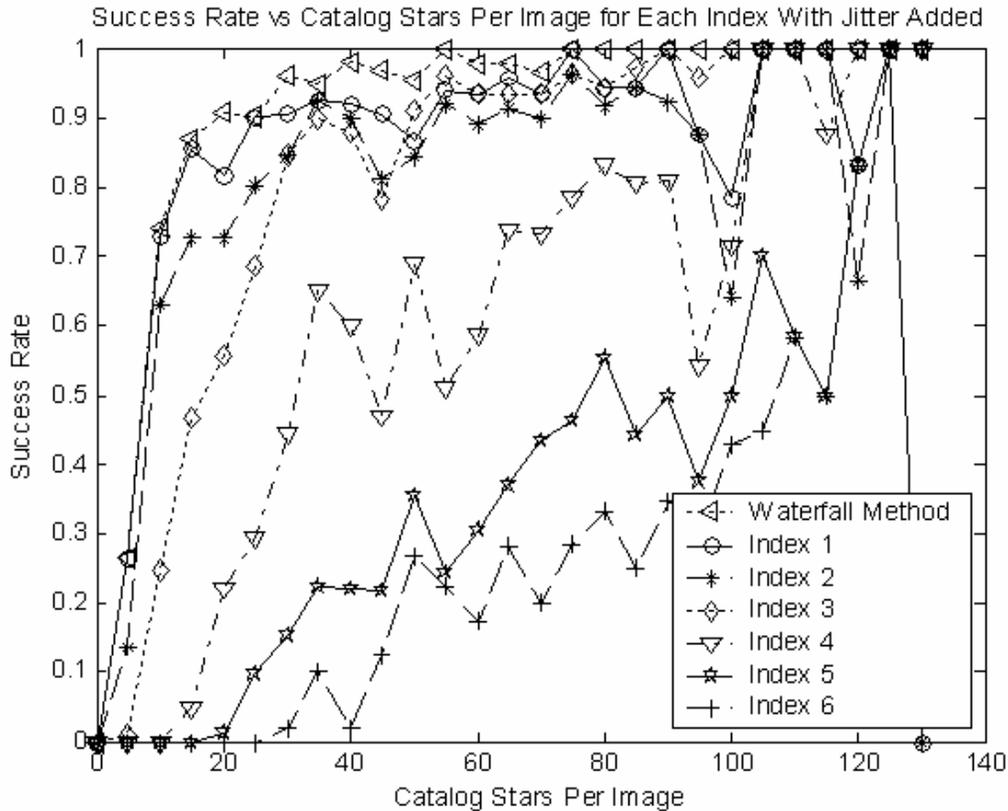
Figure 21: A plot of the change in success rate for different numbers of catalog stars per image, when positional jitter was added. The numbered indexes refer to the indexes described to at the beginning of Section 3.6. The waterfall approach refers to the process of using all the indexes together.
