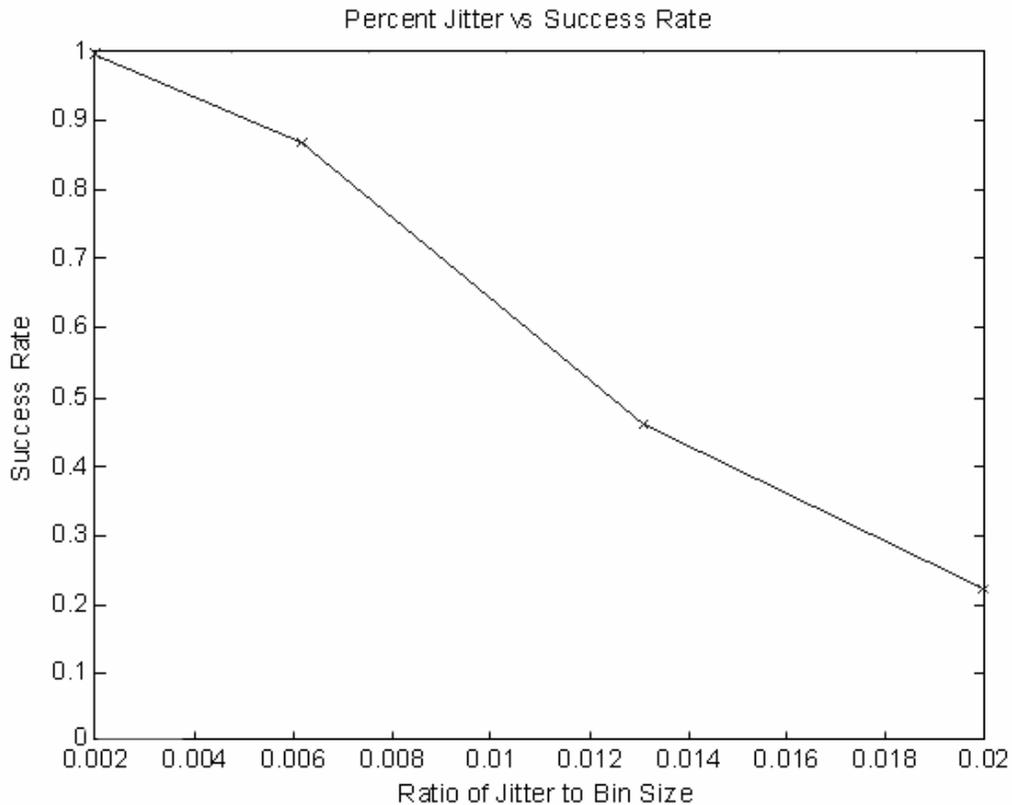
**Figure 12:** The success rate of the grid-based approach when jitter was added to the star positions, and the bins were not expanded to compensate. The ratio of jitter to bin size refers to the jitter added to the image relative to the size of the bins used to match the image.
