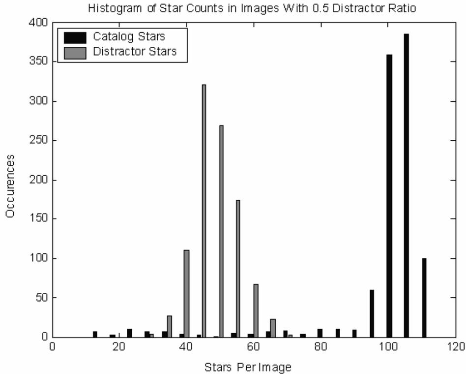
**Figure 6:** A histogram showing the distribution of the number of catalog and distractor stars present in the test images when a distractor ratio of 0.5 distractor stars for every catalog star was used.
