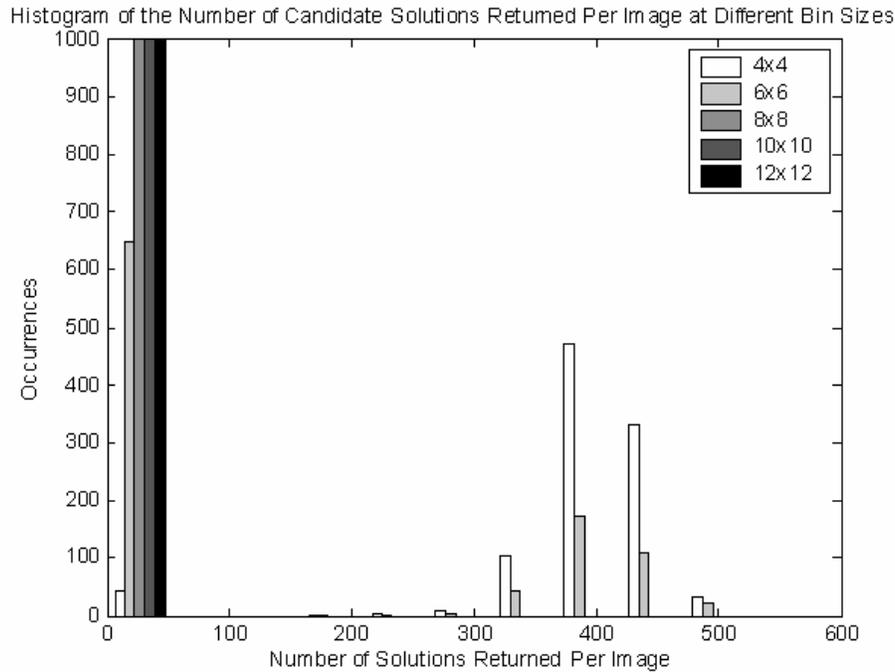
**Figure 9: The distribution of the number of solution candidates returned per image at various bin sizes. No distractors were present in the test images. Note that when the bin size was at or above 8x8 seldom more than one solution candidate was returned by the algorithm.**
