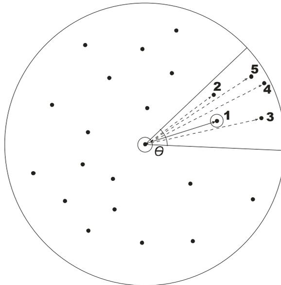
**Figure 14: An image of the initial indexing step. A wedge of angle  $\theta$  is rotated around a star, oriented using a second star (in this case the star labeled '1'). Note that the orienting star need not be the nearest star to the central star of interest.**
