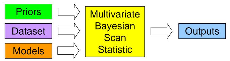
Given a set of event types  $E_k$ , a set of space-time regions S, and the multivariate dataset D, MBSS outputs the <u>posterior probability</u>  $Pr(H_1(S, E_k) | D)$  of each type of event in each region, as well as the probability of no event,  $Pr(H_0 | D)$ .
