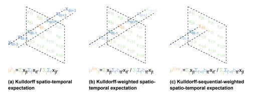
Figure 1: Illustrating the three proposed options to obtain *spatio-temporal expectations*  $\mu_{it}$  used in the computation of SPATE for single-channel data. The orange value is the current observation, the green values all other spatial units at the current time step t and all values over time at the current spatial unit i are colored blue.
