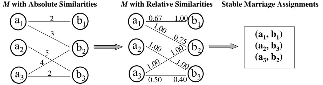
Figure 3.2: An example of a procedure for solving the stable marriage problem
