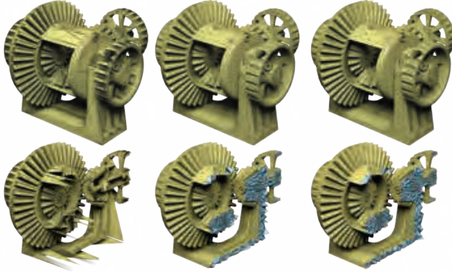
Figure 2.9: Voxel stuffing produces a tetrahedral mesh (middle) of quality comparable to a direct BSP-tree construction (right), but reduces the running times from 3292.3 seconds to 2476.6 seconds.
