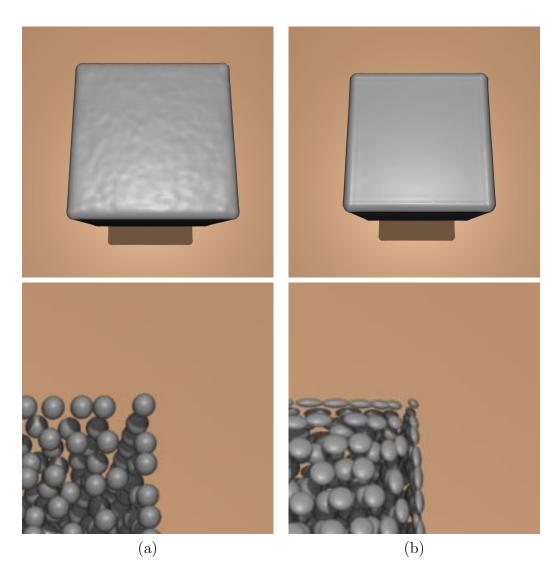
Figure 4.1: A comparison between the surface reconstruction using isotropic kernels (a) and our anisotropic kernels (b). Top row: the surface of SPH particles from a single dam break simulation. Bottom row: Illustration of particles at the top right corner. The shape of a particle in (b) represents the anisotropy of the corresponding smoothing kernel. Note that our approach constructs a flat surface with sharp edges and corners from properly stretched particles.
