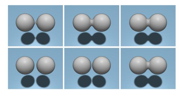
Figure 4.2: Merging spheres. Top: Not accounting for components. Bottom: Correction using connected components.
