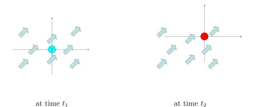
Figure 3.1: Illustration of the Lagrangian form of the material derivative. Particle p flows with the background velocity field (diagonal arrows) and a reference frame moves along with the particle. The change of the quantity  $\phi$  is represented by the change of color of the particle. As we sit on the particle, only the change on particle p is observed.
