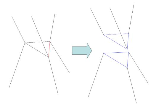
Figure 5.1: Replication of the ring edges. Left: A red colored edge is flagged for the collapse operation. Right: Instead of collapsing the edge, the mesh is separated by replicating the ring edges into the blue colored triangles.
