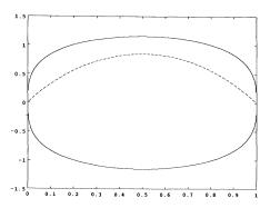
Fig. 6. Strongest hinged-hinged column and first buckling mode. p = 2,  $\alpha = 0$ .
